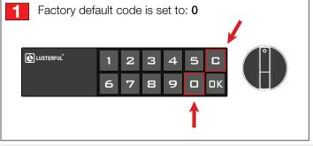
1. Type in the combination code. For first time use, code will be set as default factory code  ${\bf 0}.$  Then press  ${\bf C}.$
