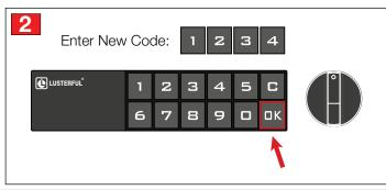
2. Type in a new 1-15 digit combination code then press  $\mathbf{OK}.$  The beep signals the new code has been set.
