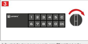
3. To unlock the door, type in your code, press  $\mathbf{OK}$  and then turn the door release  $\mathbf{clockwise.}$
